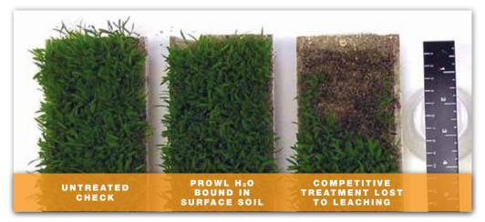
Surface application of PROWL H<sub>2</sub>O herbicide to vertical columns of Green foxtail. After 3 inches of precipitation, PROWL H<sub>2</sub>O remains bound and concentrated in the top 1 cm of surface soil.
